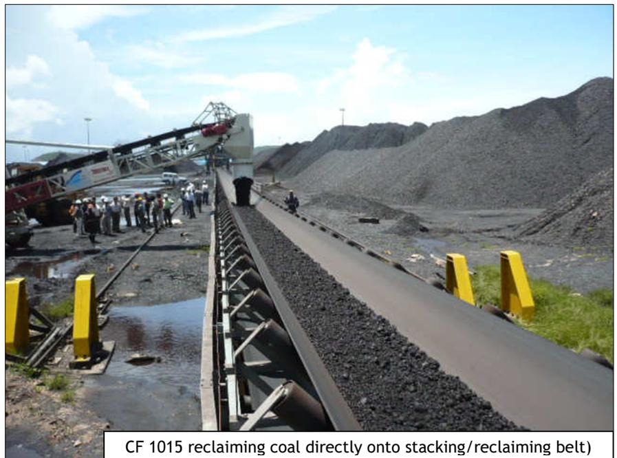
CF 1015 reclaiming coal directly onto stacking/reclaiming belt)
