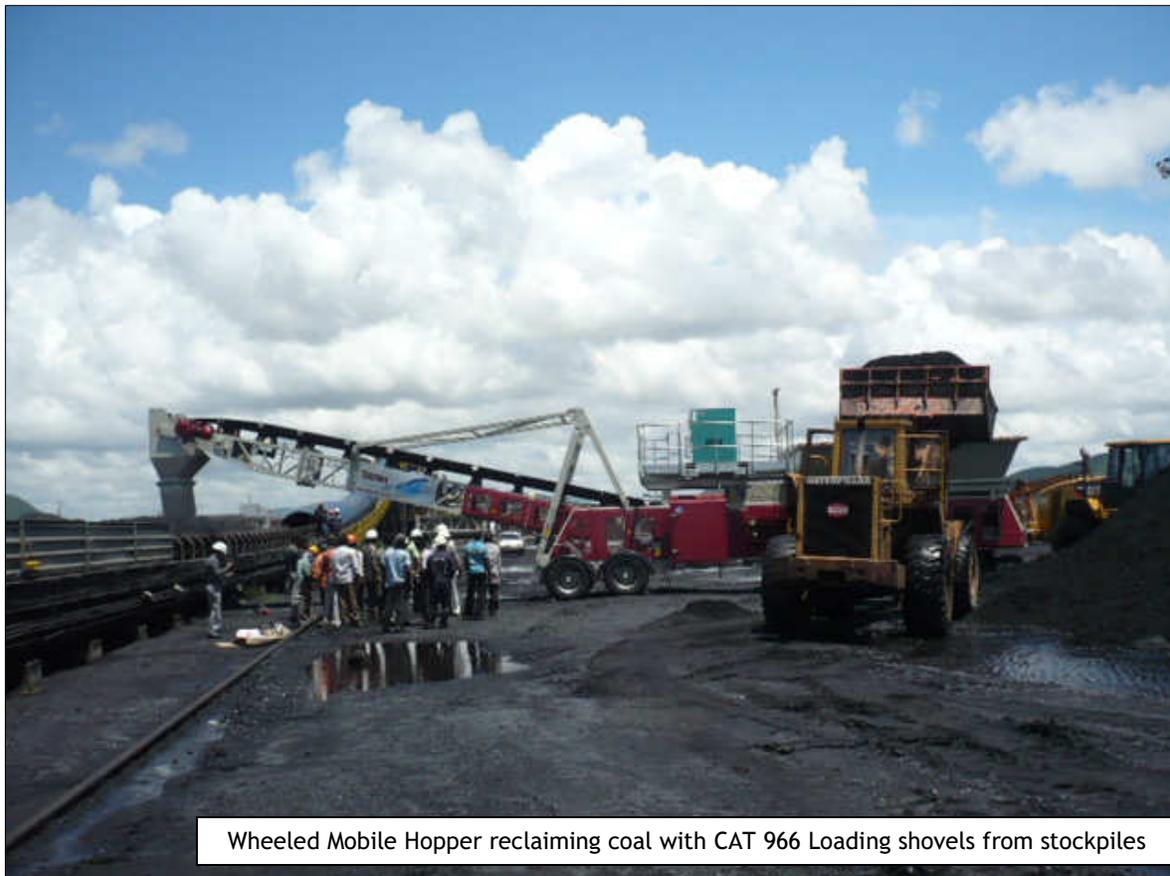
Wheeled Mobile Hopper reclaiming coal with CAT 966 Loading shovels from stockpiles
