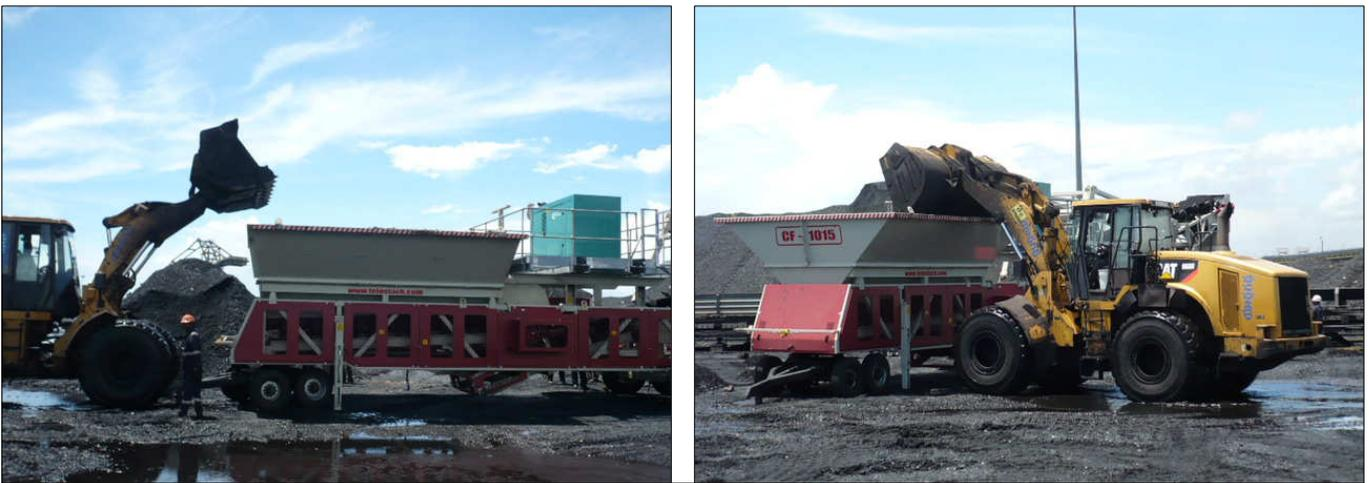
CF 1015 Wheeled Reclaim Hopper fed from CAT 966 loading shovel from 3 x sides (Left, right and rear)
