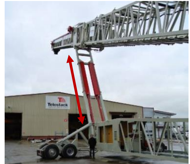
Telescopic fully lowered and retracted c/w 360 degree trimmer chute
